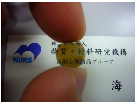
Fig. 5. Photograph of yttria stabilized zirconia disk produced by SPS at 1100 °C for 10 min under the pressure of 400 MPa. The sample was placed 30 mm above the text. The thickness of the sample is about 1 mm.
